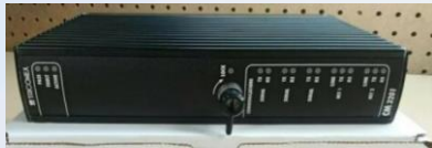
Triconex communication PLC module
