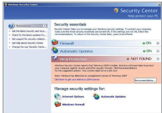
Figure 4: Screenshot of FakeXPA, the sixth most prevalent piece of malware detected by Microsoft in the first half of 2009.
